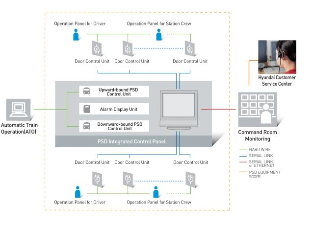
PSD NDAI Platform Screen Doors ADVANTAGE OF HYUNDAI PSD SYSTEM
